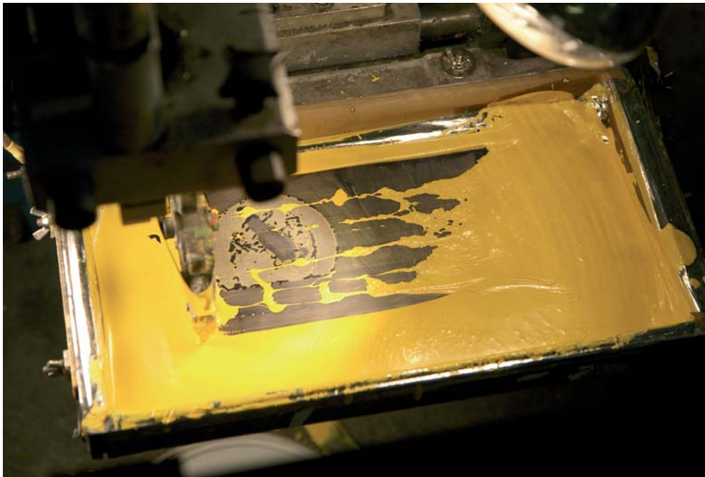
Printing in action – applying the second GBBF base colour to glassware beneath silkscreen
