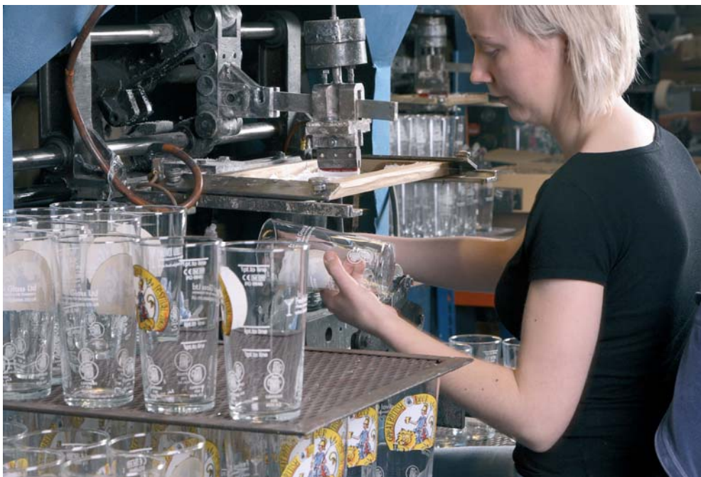
Embossed-effect – CAMRA logos are added to the bottom of GBBF glasses and stacked ready for firing in the furnace
