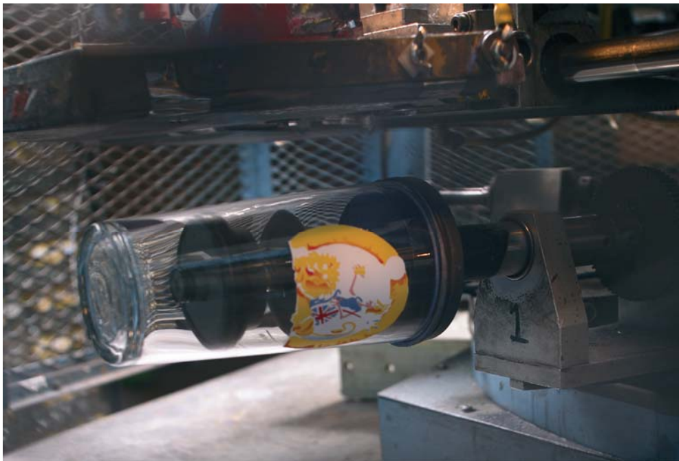
Nearing print completion – unfinished GBBF glass travels along automated print line awaiting black, final colour application
