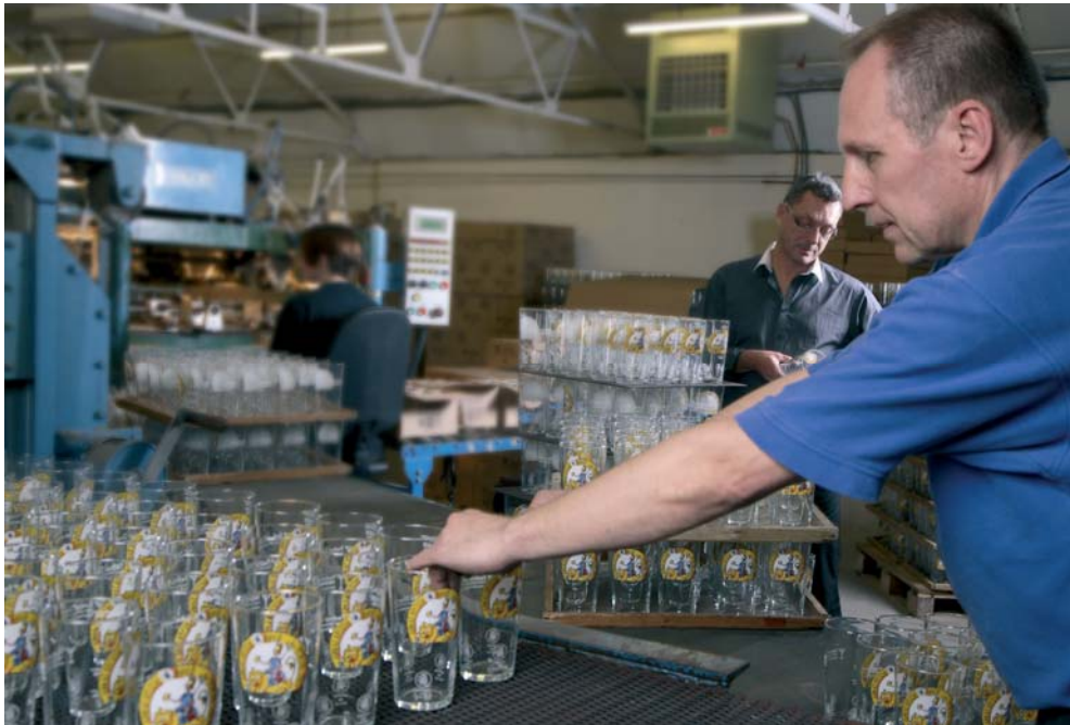
Ready for the firing – GBBF glasses are lined up on the furnace conveyor belt, with final inspection by Graham Cheesbrough, Managing Director
