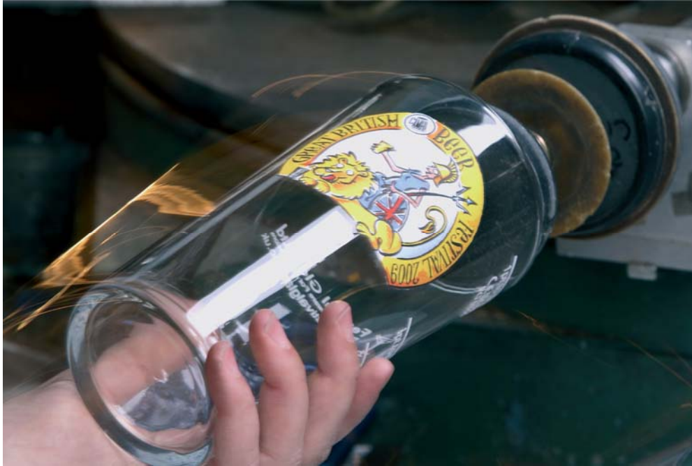
Printing complete – removing a finished GBBF from the screenprinting machine
