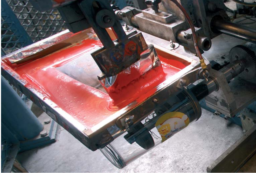
Fourth colour application – thermoplastic red ink is pulled through onto a semi-printed GBBF glass
